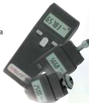
The new hand-held stroboscope measures and tests rotational and vibrational movements even in places which are difficult to access. It does this without any encroachment whatsoever in the system to be tested. When the displayed strobe frequency equals the true speed, the moving part will appear stationary.
